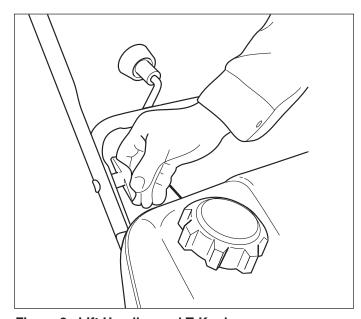
Figure 2. Lift Handles and T-Knobs
